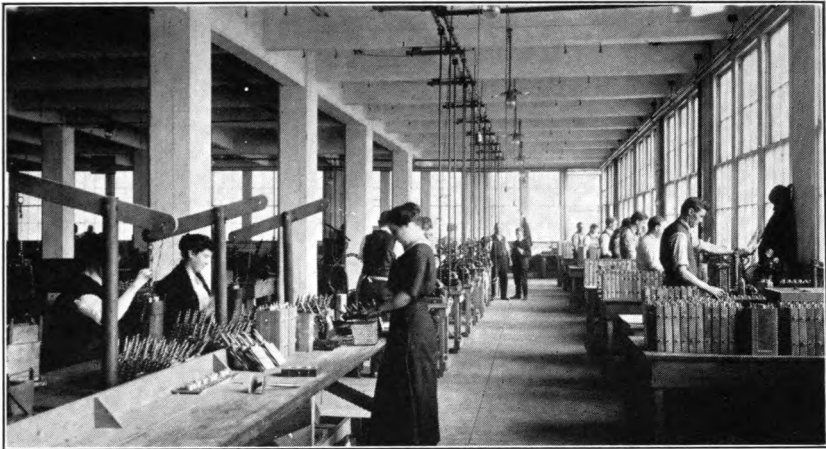
The Positive and Negative Plates are assembled on their respective pole pieces and intermeshed, after which they are assembled with special hard rubber insulators in a steel container and the top is welded on.
