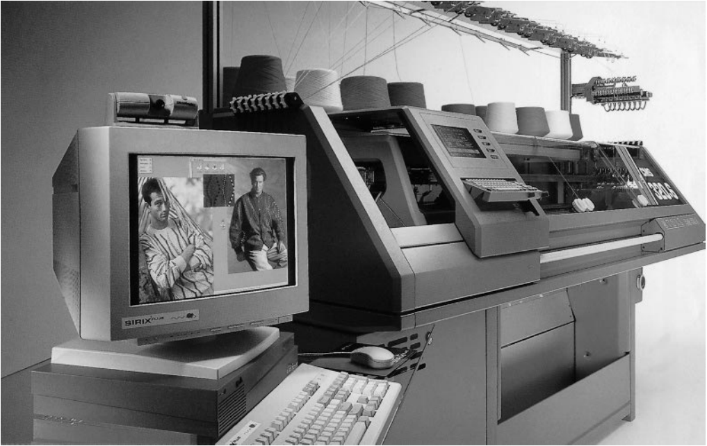
Fig. 12.2 Knitting patterns and programmes are quickly generated using automatic routines. These are checked and can be transmitted on-line to the CMS knitting machine. Simultaneous monitoring of production can also be achieved [Stoll SIRIX].
