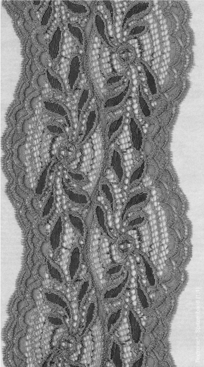
Fig. 28.16 Leaver's lace effect produced on a Textronic raschel lace machine [Karl Mayer Textronic].
