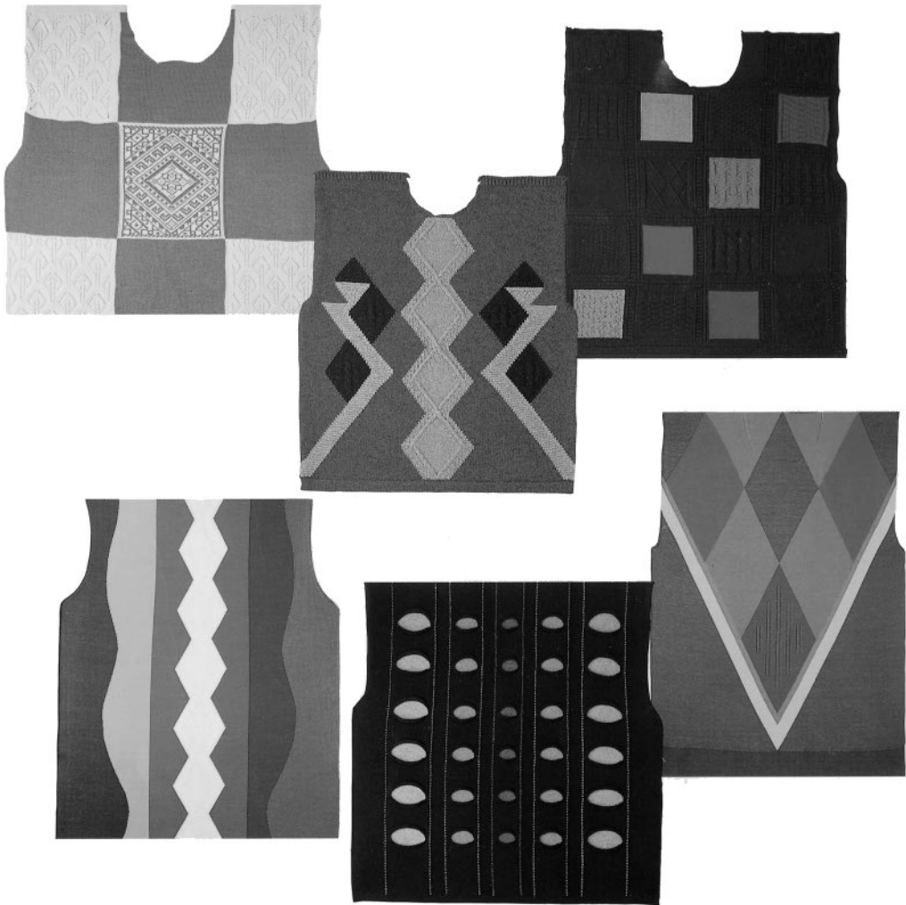
Fig. 10.3 Examples of intarsia designs knitted on an electronic V-bed machine [Shima Seiki].
