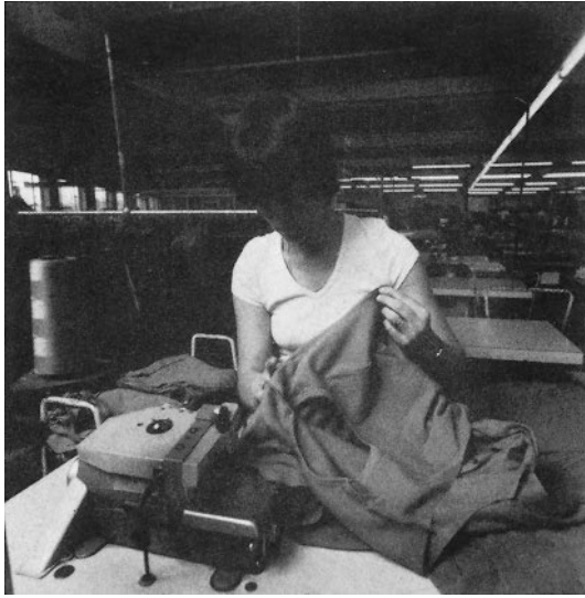
Fig. 6.3 Overlock seaming [Corah].
